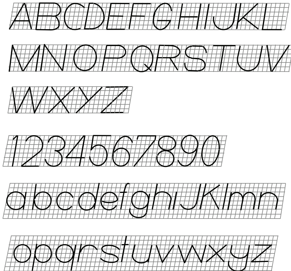
Fig. 1.18 Single stroke inclined letters and numerals.
