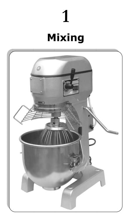
**Mixing** may be defined as a unit operation that aims to treat two or more components, initially in an unmixed or partially mixed state, so that each unit (particle, molecule etc.) of the components lies as nearly as possible in contact with a unit of each of the other components.
