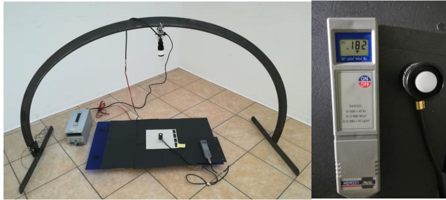
Figure 5: a) Experimental equipment for the directional reflectivity characterization; b) Photo-Radiometer Delta Ohm HD 9221 with an LP 9221/RAD probe
