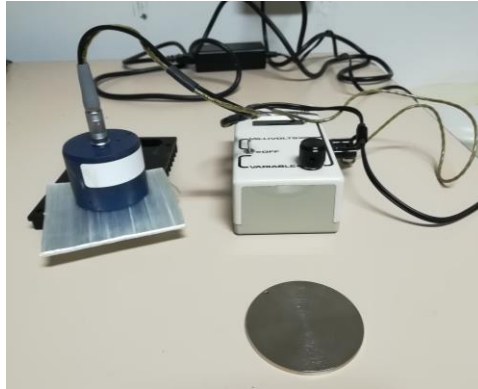
Figure 3: AE1 RD1 Emissometer D&S with Scaling Digital Voltmeter and the tested sample
