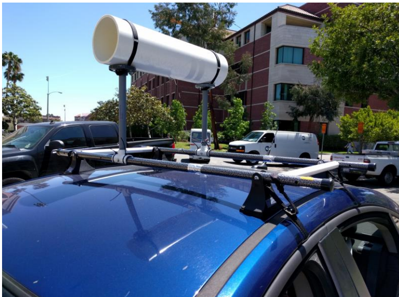
Figure 2. Mobile monitor on quick-install car-roof mount. System includes white PVC-pipe shield, gray PVC-pipe vertical risers, aluminum tube roof mounting on plastic and rubber feet, and white PVC-pipe crossbeams. Straps with hooks (not shown) secure the bars to the vehicle frame.
